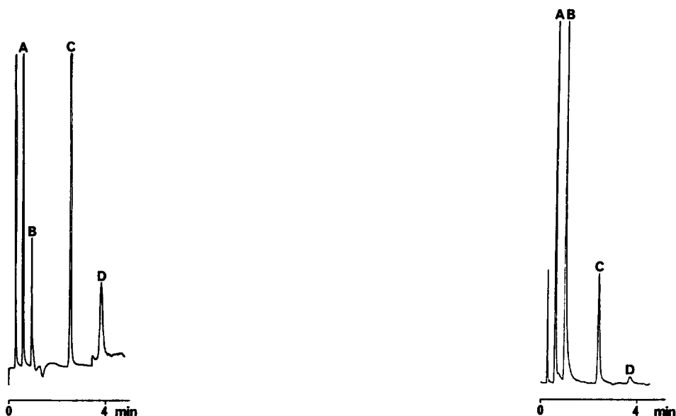
Fig. 2. UV trace (215 nm, range 0.1 a.u.f.s. for 3.5 min then range 0.01 a.u.f.s.) obtained from SFC of a mixture of (A) levamisole, (B) furazolidone, (C) chloramphenicol, and (D) lincomycin on a 100 \times 4.6 mm I.D. column packed with 5\text{-}\mu\text{m} amino-bonded Spherisorb. The mobile phase was carbon dioxide modified with 15% methanol at a flow-rate of 4 ml/min. Column pressure 351 bar; temperature 75^\circ\text{C} .
